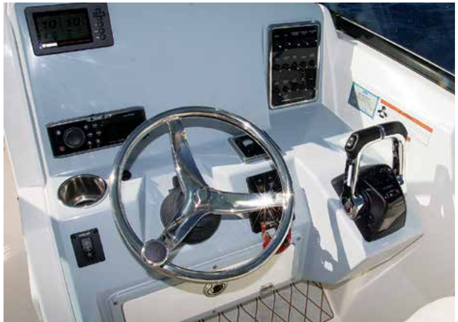
The helm station on the starboard console features a tilt-and-lock wheel, glove box, angled footrest and room for a flush-mounted 12-inch multifunction display.
