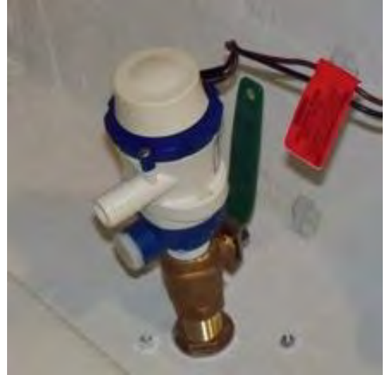
Livewell Pump Assembly in the “OPEN” Position
