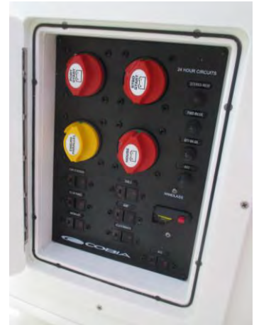
Battery Switch (Shown in the Off Position)
