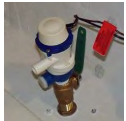
Livewell Pump Assembly in the “OPEN” Position
